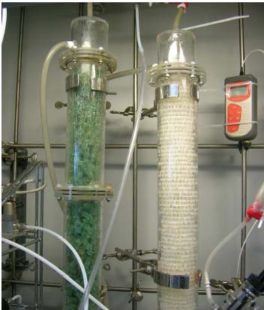
Fig. 3a and 3b Laboratory trickling filter for biological siloxane cleaning at Profactor GmbH and combined trickling filter for H 2 S and siloxane cleaning at biogas plant in Frieres
