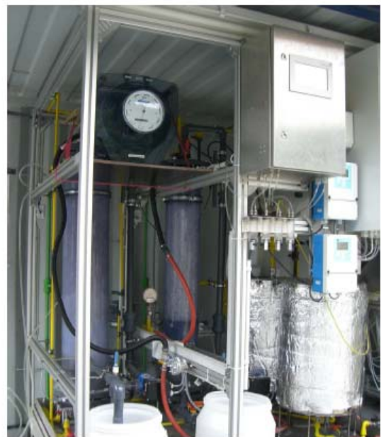
Fig. 3a and 3b Laboratory trickling filter for biological siloxane cleaning at Profactor GmbH and combined trickling filter for H 2 S and siloxane cleaning at biogas plant in Frieres
